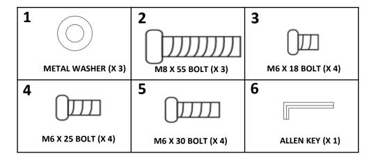
STEP 1: Open Velcro flap on bottom of seat (B) and align the holes with those found on the seatback (A). Pass each M8x55 bolt (2) though a metal washer (1) and insert into aligned bolt holes. Tighten with Allen Key (6). "CHAIR SEAT" COMPLETE
